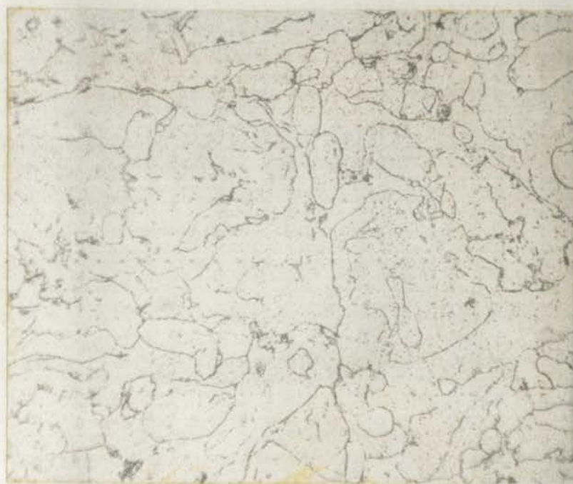
Figure 6. Micrograph showing the cross-sectional appearance of densified plasma-sprayed 1100 aluminum, etched, 250X.
