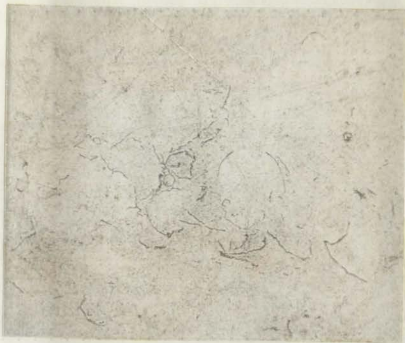
Figure 5. Micrograph showing the cross-sectional appearance of densified plasma-sprayed 1100 aluminum, 250X.
